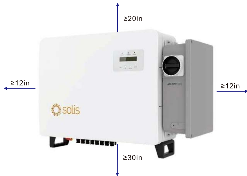
Figure 3.2 Clearance distances requirement for the inverter
