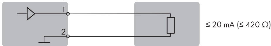
Figure 10: Connection of an analog remote terminal
